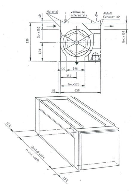
Working width 1000 / 1250 / 1500 / 2000 / 2500 mm The AFS is used for air and dust separation. Special working widths are also available on request. The necessary connecting pieces are available as special accessories.
